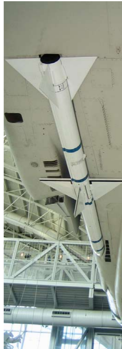
Sparrow missile under a Phantom aircraft. Photo courtesy of Dr A. Neely
