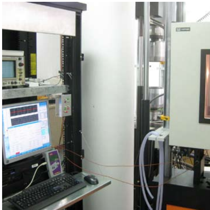
High-strength Aerospace-grade aluminium undergoing fatigue testing at 150°C
