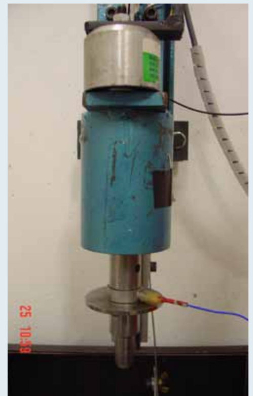
Set-up for impact testing
